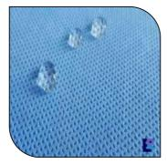
PP (Polypropylene) laminated non-woven fabrics are a type of composite material made by laminating a layer of polypropylene film to a layer of non-woven fabric.
